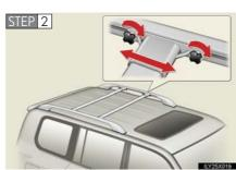
Slide the cross rails to the appropriate position for loading luggage and turn the knobs clockwise to tighten the cross rails securely.
