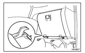
(b) Remove the 2 screws and glove compartment door as shown in the illustration.
