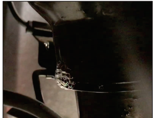
Figure 4. Example of Results if Leak is Present
