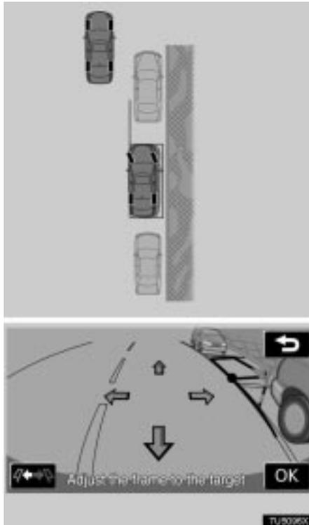
The assisted parking position will be closer to the middle of the road (further from the shoulder) than the set target parking position.
