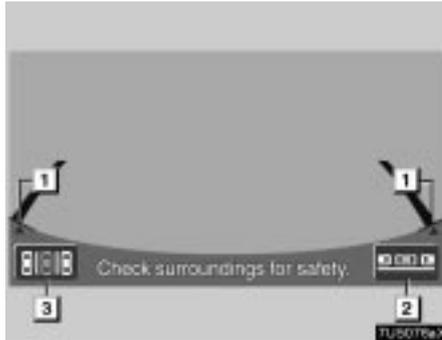
**To activate the advanced parking guidance system, place the selector lever in “R” position when the engine switch is in “IG-ON” mode.**
