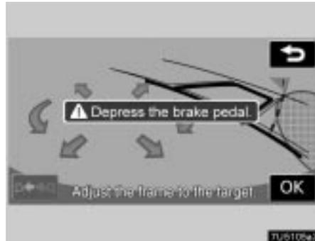
This screen will be displayed when “OK” is touched while the brake hold system is on.
