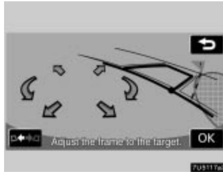
When in the parking assist mode, if the message "Steer to right (of left) until the frame becomes green." is displayed, you may use the assist mode by turning the steering wheel.
