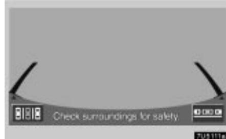
8. Once the vehicle is mostly within the target parking position, voice guidance will give the message "The guidance is finished" and parking assist mode will finish.
