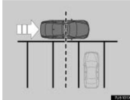
If no vehicle or small vehicles are parked on both sides of the desired parking space, stop with the steering wheel straight.
