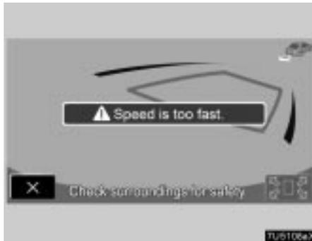
If the vehicle's backing up speed is too fast, a warning tone will sound. If you continue to back up at that speed, the system will be disabled. Back up at a speed that does not cause the warning tone to sound. The green frame displayed on the screen is approximately the same size as your vehicle. (The green frame displayed when setting the target parking position is the size of a normal parking space.)
