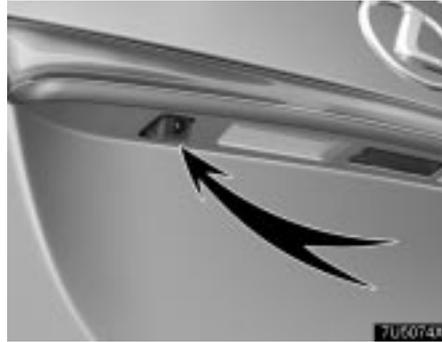
The advanced parking guidance system camera is located on the trunk as shown in the illustration.
