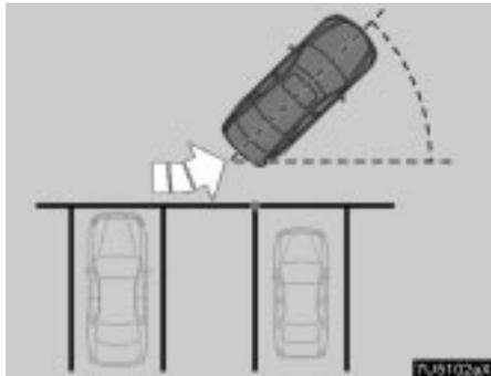
3. Position your vehicle so that you can enter the parking space, then stop the vehicle with the steering wheel straight.
