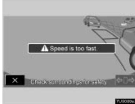
If the vehicle's backing up speed is too fast, a warning tone will sound. If you continue to back up at that speed, the system will be disabled. Back up at a speed that does not cause the warning tone to sound.
