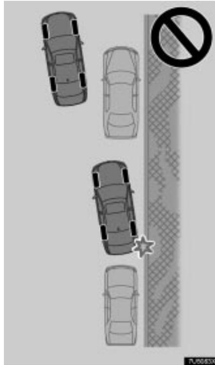
2. Stop your vehicle in a position where you can see the front edge of the leading parked vehicle right beside you, with the steering wheel straight.
