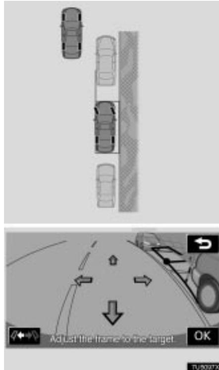
In this case, if you align the warning flag with the rear of the forward parked vehicle, and the green extension guide line with the lower edge of the parked vehicle's rear wheel when setting the target parking position, the left side of your vehicle will be roughly in line with the left side of the front parked vehicle once assisted parking is complete. If you are parallel parking on the opposite side of the road, left and right will be reversed.
