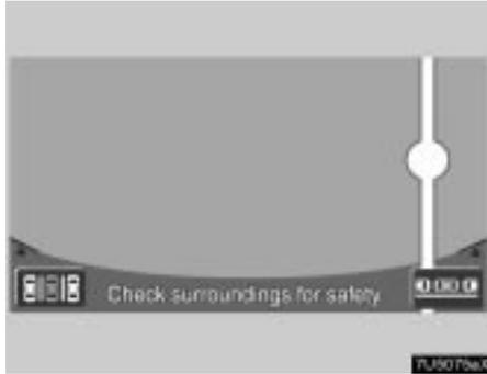
If a bright light (for example, sunlight reflected off the vehicle body) is picked up by the camera, the smear effect\*, peculiar to the CCD camera, may occur.
