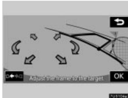
6. Use the arrow to align the green frame with the desired parking space, then touch "OK".
