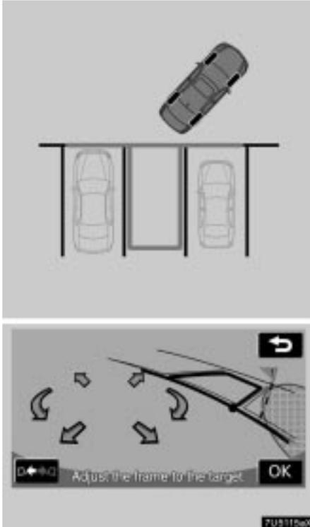
If the lines of the parking space are wider than the green frame, position the frame so that the difference between the frame and the parking space lines is equal on both sides.
