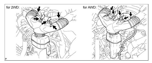
**b.** Install the intake air connector pipe with the 3 hose clamps.
