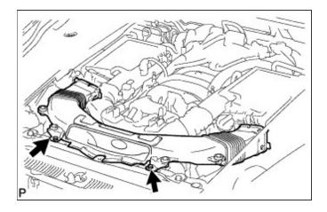
**b.** Hold the air cleaner inlet by the protrusions A and B, and detach the
