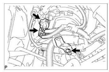
**c.** Remove the 3 bolts and camshaft timing control with EDU motor.
