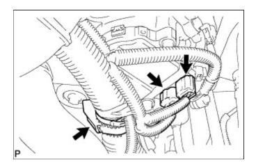
**b.** Remove the 3 bolts and camshaft timing control with EDU motor.
