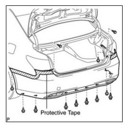
(a) Put protective tape around the rear bumper assembly.
