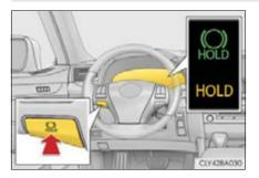
Turns the brake hold system on
