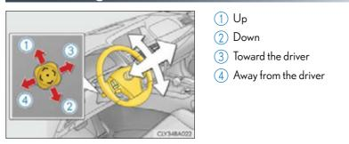
The steering wheel and driver's seat move in accordance with engine switch mode and the driver's seat belt condition. ( $\rightarrow$ P.27)
