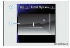
When another screen is displayed on the main display while the Lexus night view is being shown on the main display, the Lexus night view screen will be displayed on the side display.
