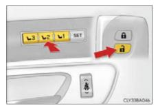
While pressing the desired switch ("1", "2" or "3"), press on the wireless remote control until the buzzer sounds.
