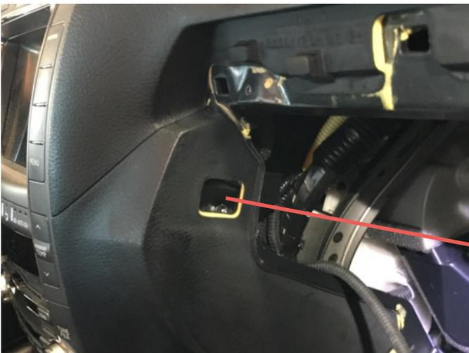
1 bolt accessed through this hole holds in the Nav unit. There's another bolt in the identical position on the opposite side which is located behind the trim panel underneath the start button.
