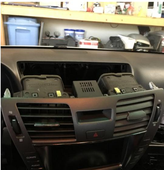
With the nav unit out of the car, you can remove the HDD by removing the 2 tamper proof torx screws and then pulling the drive out.
