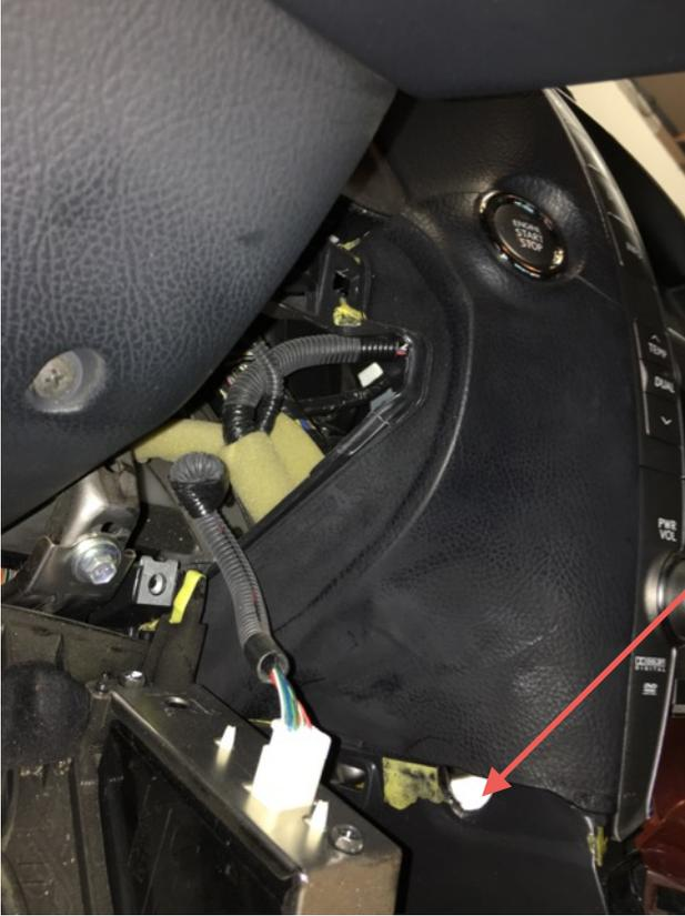
1 of 2 bolts securing the cd changer is located through this hole. There's another bolt (10mm Socket) on the opposite side same location.
