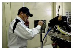
For Fujita, rigorous inspections such as checking the block and cylinder-head interiors via X-ray and CAT scan were not enough to yield the sound qualities desired of the LS. He personally fires up every assembled engine on a test bench and listens intently with a stethoscope to detect even faint variations in sound. When Fujita discovers an off-key note, he
