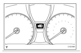
(e) Move the shift lever to the D position, and quickly move back and forth between N and D (once per less than 1.5 seconds) for at least 6 seconds.
