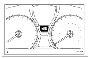
(i) When the indicator light (D) turns on, lift the vehicle up immediately.
