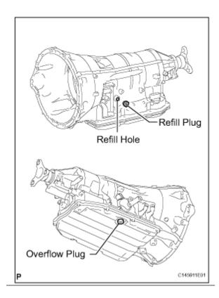
(j) Remove the overflow plug. At the proper fluid inspection temperature, check the fluid amount. If the ATF flows from the overflow tube and the ATF flows in a thin stream, the fluid amount is normal. If the ATF does not flow from the overflow tube, add ATF into the refill hole until ATF flows from the overflow tube. If the ATF flows in a thin stream, the fluid amount is normal.
