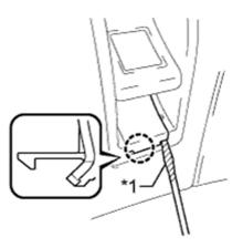
**a.** Using a screwdriver, detach the claw and remove the switch base hole cover from the No. 1 instrument panel safety pad sub-assembly.
