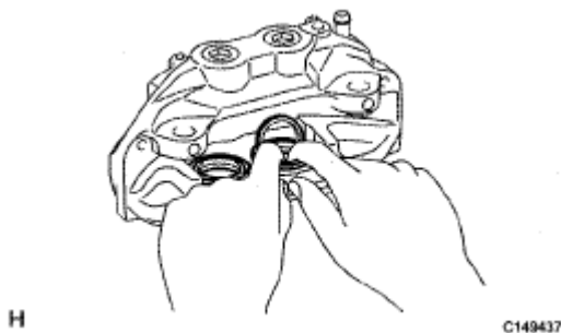
Fig. 95: Identifying Piston Seals
