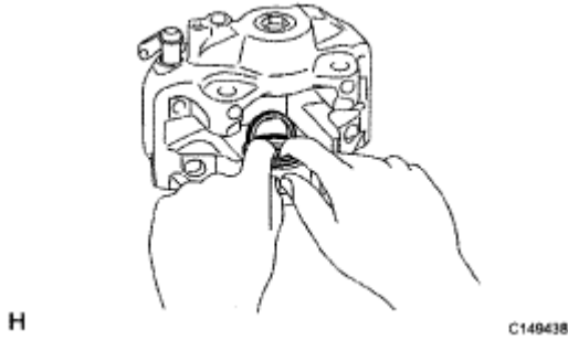
Fig. 130: Identifying Piston Seals & Disc Brake Caliper Courtesy of TOYOTA MOTOR SALES, U.S.A., INC.
