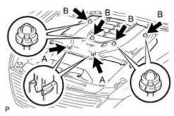
(a) While using both hands, lift the rear side of the cover upwards to detach the 4 clips B. Slide the cover towards the front of the vehicle to detach the 2 clips labeled A, and remove the V-bank cover.
