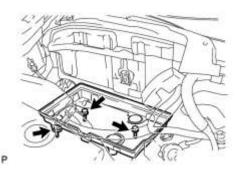
(a) Remove the 3 bolts and battery tray.
