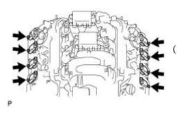
(a) Disconnect the 8 ignition coil connectors.
