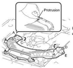
(b) Hold the air cleaner inlet by the protrusions A and B, and detach the connections.
