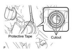
(c) Using a screwdriver, pry at the cutouts to remove the 8 ignition coils together with the 8 spark plug tube gaskets.
