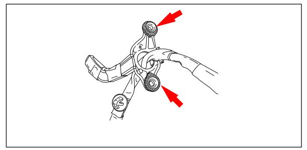
**Repair** 9. Install the outside rear view mirror assembly:
