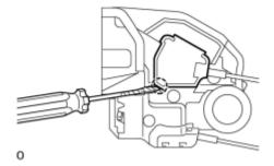
(a) Using a screwdriver, disengage the claw.
