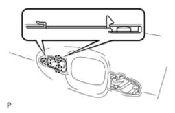
(a) Detach the 3 claws and remove the pad.
