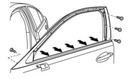
(f) Loosen the 5 belt line screws indicated by the arrows in the illustration.
