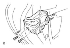
(2) Using a T30 "TORX" wrench, remove the 3 screws and door lock.
