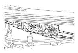
(a) Detach the claw, disconnect the connector and then remove the light.
