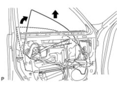
(f) Remove the door glass in the direction indicated by the arrows in the illustration.
