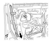
(a) Remove the 2 bolts and frame rear lower.
