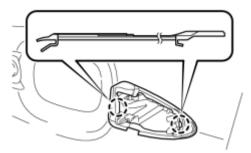
(a) Detach the 2 claws and remove the pad.
