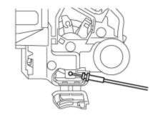
(b) Remove the front door inside locking cable assembly.
