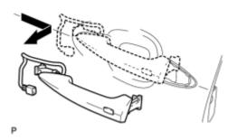
(c) Remove the handle by sliding and pulling it in the direction indicated by the arrow in the illustration.
