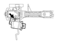
(a) Remove the screw and door electrical key oscillator.
