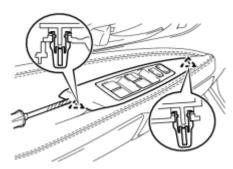
(a) Using a screwdriver, disengage the 2 clips.
