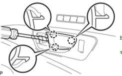
(a) Using a screwdriver, detach the 3 claws and remove the bezel plug.
