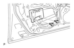
(a) Remove the 2 bolts and frame garnish pad.
