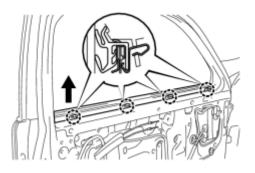
(a) Remove the weatherstrip inner by pulling it upward in the direction indicated by the arrow in the illustration.
