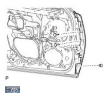
(a) Remove the 3 clips and weatherstrip from the door.
