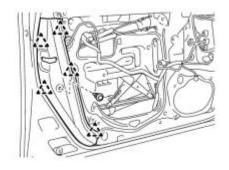
(b) Using a clip remover, detach the 5 clips.
