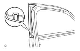
(a) Remove the 2clips and front door belt moulding end cover.
