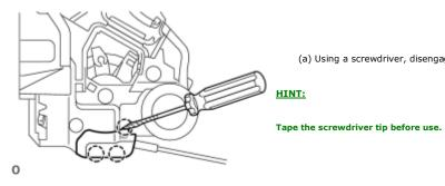
(a) Using a screwdriver, disengage the 3 claws.
