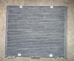
3. Push on the 3 tabs found on the front of the filter frame and lift frame up. Slide frame outwards to remove.
