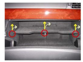
1.The filter is located behind the glove compartment. Open compartment and remove the t-shaped shelf in the glove box by lifting and pulling out the 3 retaining tabs securing the shelf. Remove shelf and set it aside.
