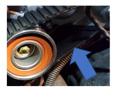
31. Remove the water pump. I pried gently in the corner by a tab. Coolant will likely come out, be ready to catch the drips.
