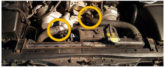
7. Disconnect the electrical clip from the radiator and unclip it from the 3 wire ties. They work like zip ties.
