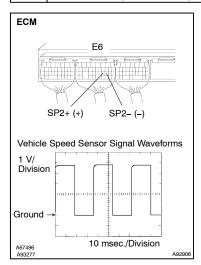
(a) Check the waveform of the ECM when the vehicle speed is approximately 60 km/h (37 mph).
