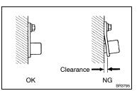
(a) Check the sensor installation.OK: Sensor is installed correctly.
