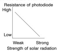
A photodiode in the A/C solar sensor detects solar radiation and sends signals to the A/C amplifier.
