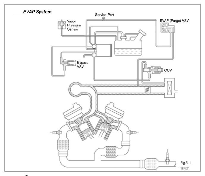
**Overview** There are a variety of EVAP systems in use with different monitoring strategies. It is essential that the EVAP system be correctly identified before beginning diagnosis (the Repair Manual is the best source). The following information covers the different systems.
