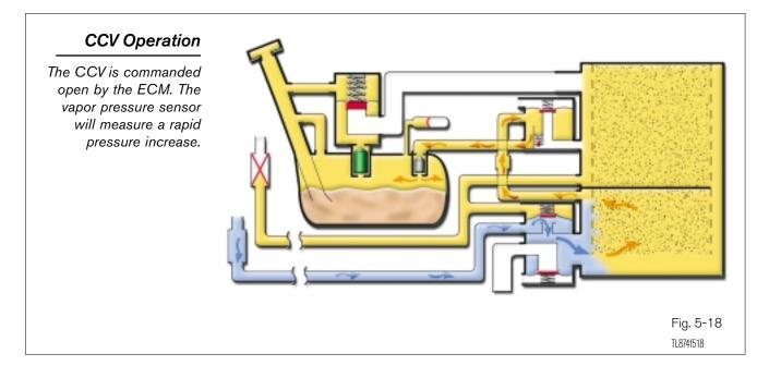
P0446:This stage checks the CCV and vent (air inlet side) operation. When the<br/>vapor pressure rises to a specified point, the ECM opens the CCV.Vent Control,<br/>CCV OperationPressure will increase rapidly because of the air allowed into the system.and Bypass VSV<br/>OperationNo increase or an increase below specified rate of pressure increase<br/>indicates a restriction on the air inlet side.
