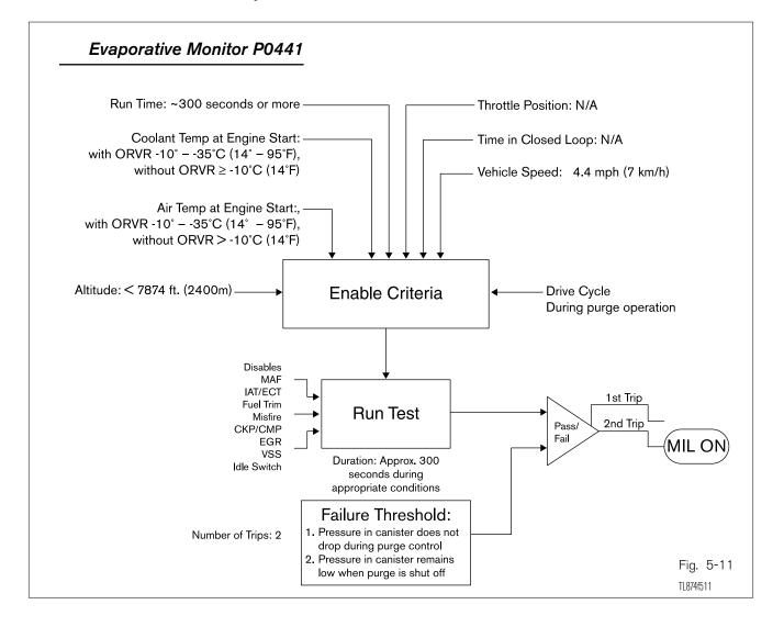
Restricted Vapor Purge Flow During purging under normal conditions, pressure pulsations are generated by the cycling of the purge VSV and canister pressure drops. If the VP sensor does NOT detect these pulsations and pressure drop in the canister, the ECM determines the EVAP system is not working. Possible causes are, the purge VSV is stuck closed, a restricted purge line, a hole or disconnected purge line.
