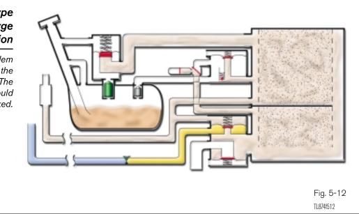
P0446: If DTC P0446 is present, a leak present on the canister purge side may Stree-Way VSV set this code.
