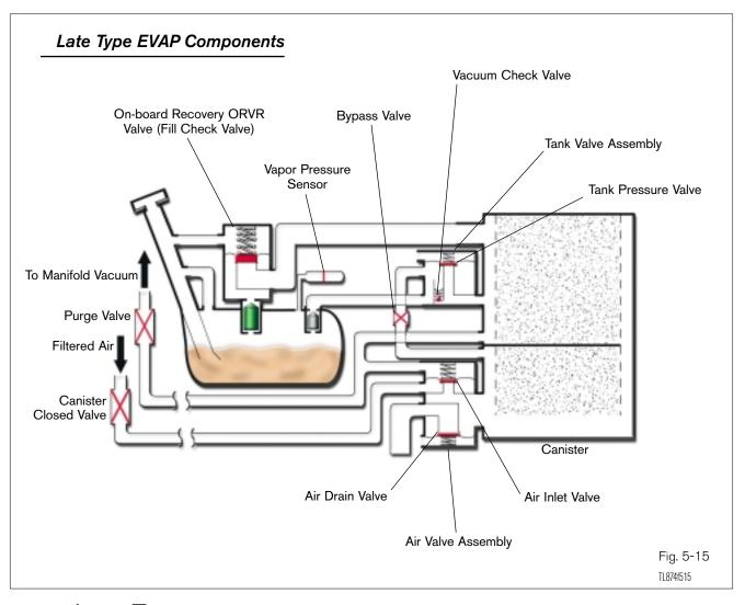
Late Type The late type, also known as intrusive type, was developed to meet the (Intrusive) wery stringent, mandated standard of detecting a hole 5mm (0.020<sup>°</sup>). This system uses many of the same components as the early type. Purge, vacuum relief, pressure relief, and ORVR operations are identical to the early type. However, the following items have been changed:
