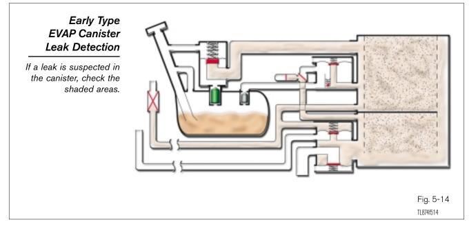
The three-way VSV is connected to the VP sensor, canister, and fuel tank. This VSV allows the VP sensor to detect either canister or tank pressure.
