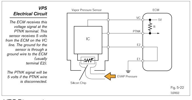
VPS Diagnosis Check all hoses for proper connection, restrictions, and leaks. Check the VC and E2 voltages. Apply the specified pressure and read sensor voltage output. The vapor pressure sensor is calibrated for the pressures found in the EVAP system, so apply only the specified amount to prevent damaging the sensor.
