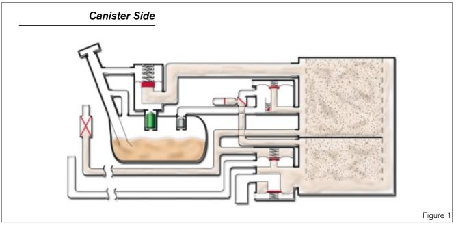
1. With the system pressurized, check shaded areas for leaks (soapy water detection).
