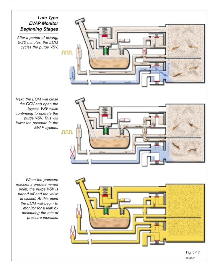
**PO441:** At a predetermined point, the ECM closes the CCV and opens the Purge VSV bypass VSV causing a pressure drop in the entire EVAP system. Operation The ECM continues to operate the purge valve until the pressure is lowered to a specified point at which time the ECM closes the purge valve. If the pressure did not drop, or if the drop in pressure decreased beyond the specified limit, the ECM judges the purge VSV and related components to be faulty.
