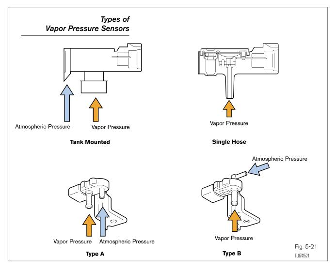
Vapor Pressure Sensors come in a variety of configurations. When the VPS is mounted directly on the fuel pump assembly, no hoses are required. For remote locations, there may be one or two hoses connected to the VPS. If the VPS uses one hose, the hose is connected to vapor pressure. In the two hose configuration, one hose is connected to vapor pressure, the other hose to atmospheric pressure. It is important that these hoses are connected to the proper port. If they are reversed, DTCs will set.
