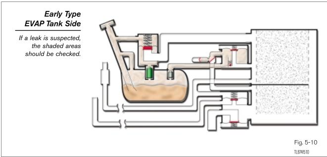
P0441:The EVAP monitor is designed to detect:Vapor PurgeFlow Detection• restricted vapor purge flow when the purge VSV is open
