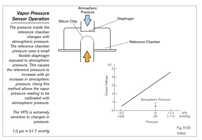
This sensor uses a silicon chip with a calibrated reference pressure on one side of the chip. The other side of the chip is exposed to vapor pressure. Changes in vapor pressure cause the chip to flex and vary the voltage signal to the ECM. The voltage signal out depends on the difference between atmospheric pressure and vapor pressure. As vapor pressure increases, the voltage signal increases. This sensor is sensitive to very small pressure changes (1.0 psi = 51.7 mmHg).
