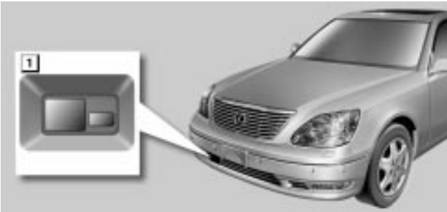
► Dynamic laser cruise control (Vehicles without pre-collision safety system) ① Laser radar sensor
