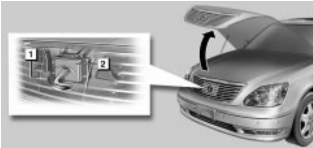
► Dynamic radar cruise control (Vehicles with pre-collision safety system) ① Millimeter wave grille cover ② Millimeter wave radar sensor
