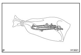
(c) Put the removed curtain shield airbag in a clear plastic bag and keep it in a safe place.
