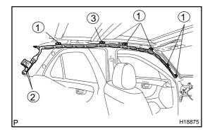
(b) In the order shown in the illustration, remove the bolts and curtain shield airbag assembly.
