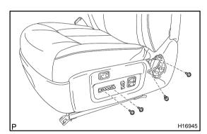
5. **REMOVE FRONT SEAT CUSHION SHIELD** Remove the 4 screws and front seat cushion shield.
