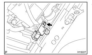
4. REMOVE SEAT POSITION SENSOR ASSEMBLY
