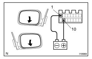
(d) Revese the polarity, and check that the mirror turns downward.
