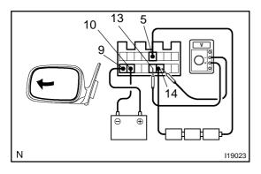
Apply battery positive voltage to terminals 9 and 10, then (g) the table below while the mirror moves between the leftmost position and right-most position.
