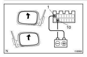
(c) Connect the positive (+) lead from the battery to terminal 1 and the negative (–) lead to terminal 10, and check that the mirror turns upward.
