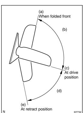
(2) Reverse the polarity, check that the mirror does not operate.
