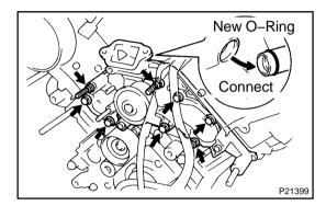
(b) Install a new O-ring to the water bypass pipe end.
