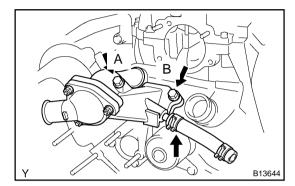
(g) Install the water inlet and housing assembly with the 2 bolts. Alternately tighten the bolts.
