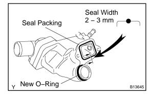
(b) Apply seal packing to the sealing groove of water inlet housing as shown in the illustration.
