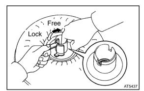
(b) Press on the serrations of starter with a finger and rotate
