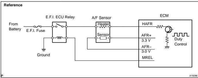
To obtain a high purification rate for the CO, HC and NOx components of the exhaust gas, a three–way catalytic converter is used, but for the most efficient use of the three–way catalytic converter, the air–fuel ratio must be precisely controlled so that it is always close to the stoichiometric air–fuel ratio.
