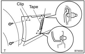
(e) w/o Mudguard: Using a hexagon wrench, install the 2 screws.
