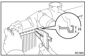
(b) Check the lock plate height (H) after completing the caulking.
