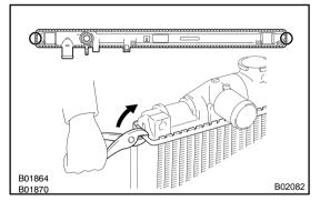
The points shown in the illustration cannot be staked with the SST. Use pliers or similar object and be careful not to damage the core plates.
