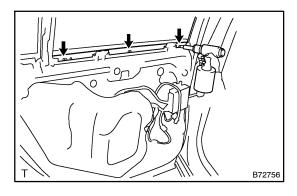
(b) Using a hand riveter or an air riveter, install the glass run to the door with the 3 rivets.
