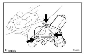
Using a T25 torx® driver, remove the 3 screws and motor. (b)
