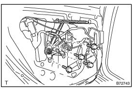
(b) Install the window regulator with the 4 bolts.
