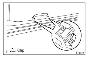
(i) Using a screwdriver, disengage the 2 clips and remove the courtesy lamp.
