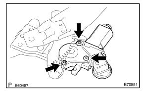
(b) Using a T25 torx<sup>®</sup> driver, install the motor with the 3 screws.
