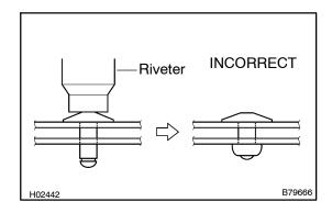
Do not have any space between the glass runs. Firmly hold together the 2 items while installing the rivet.
