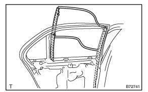
(d) Remove the glass run as shown in the illustration.
