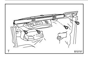
(h) w/ Rear side curtain:Remove the 4 screws and curtain.
