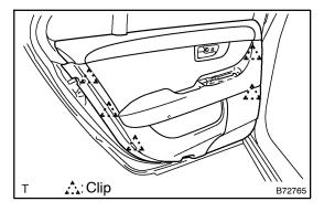
(b) Using a screwdriver, disengage the 5 clips and remove the trim.
