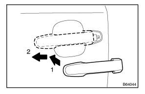
(c) Install the handle by pushing it in the direction indicated by the arrow marks in the illustration.
