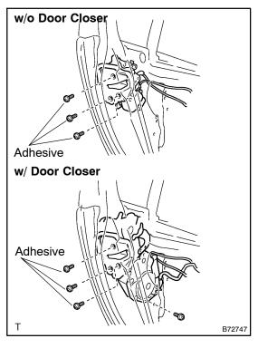
(b) Apply adhesive to the threads of the 3 screws.
