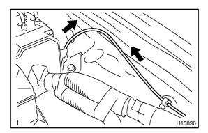
(b) Pull the cable from the engine room to remove it.
