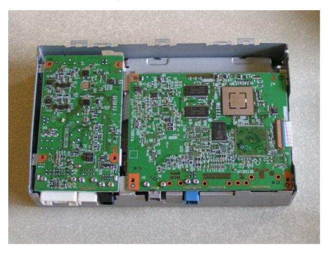
Flip over the left circuitboard on the picture, and press the switch for several seconds.
