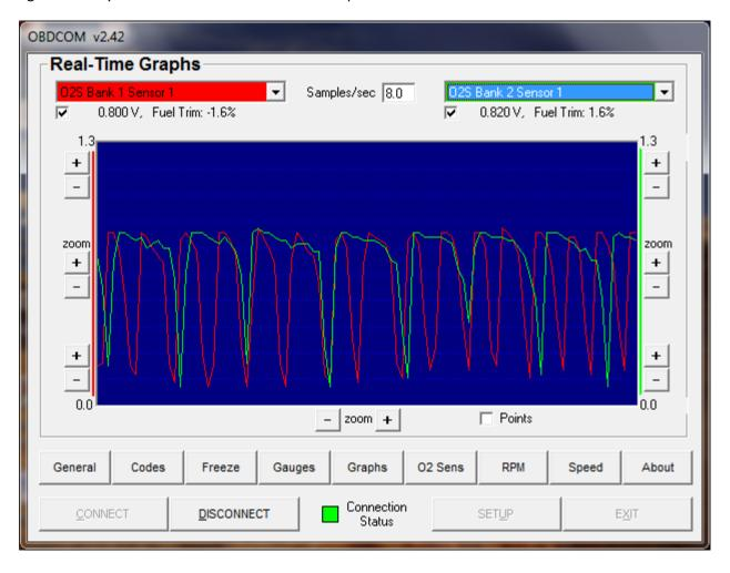
Bank 1 O2 sensors pre (Sensor 1) and post (sensor 2) catalytic converter. Note that sensor 2 is much dampened suggesting catalytic converter is doing its job of absorbing and releasing O2 from exhaust.
