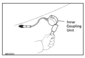
(c) Using a scraper or screw driver, remove inner coupling unit from back window glass.
