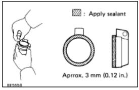
(c) Remove the protective paper from the outer coupling unit and apply sealant in plenty to the bottom surface of the coupling unit as shown in the figure.
