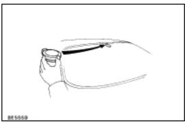
(d) Adhere the outer coupling unit strongly against the installation location until the entire double–sided tape comes in contact with the glass and the sealant comes out.
