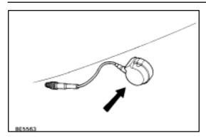
(c) Install the inner coupling unit to the glass.
