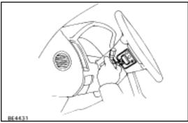
(b) Install the commande module and a screw.
