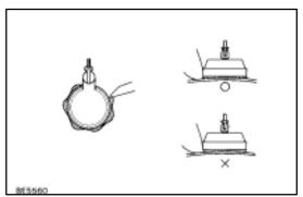
(e) Using a scraper or spatula, remove excess sealant.
