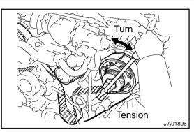
(c) Turn the LH camshaft timing pulley counterclockwise until there is tension between the crankshaft timing pulley and LH camshaft timing pulley.
