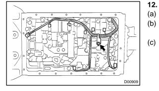
Install the 21 bolts. Torque: 10 N·m (100 kgf·cm, 7 ft·lbf) **Bolt length:** Bolt A: 23 mm (0.91 in.) Bolt B: 28 mm (1.10 in.) Bolt C: 36 mm (1.42 in.) Bolt D: 55 mm (2.17 in.)
