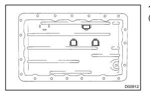
(b) Install the oil strainer with the 4 bolts. Torque: 10 N·m (100 kgf·cm, 7 ft·lbf)
