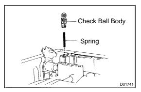
7. REMOVE CHECK BALL BODY AND SPRING NOTICE: Do not drop the check ball body and spring.
