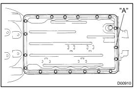
(d) Install the oil pan with the 19 bolts. **Torque: 7.4 N·m (75 kgf·cm, 65 in.·lbf)**
