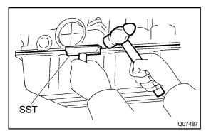
(b) Install the blade of SST between the transmission case on oil pan, cut off applied sealer, and remove the oil pan. SST 09032 – 00100
