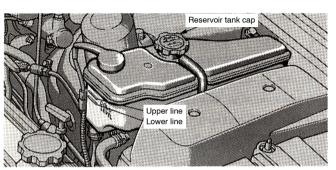
Park the vehicle at a level spot and look at the see through coolant reservoir tank when the engine is cool. The coolant level is satisfactory if it is between the upper and lower lines on the tank. If the level is low, add ethylene-glycol type coolant.
