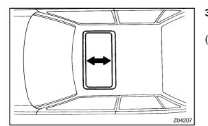
2. ADJUST SLIDING ROOF GLASS LEVEL DIFFERENCE Using a torx driver, adjust the level difference by tightening or loosening the bolts.
