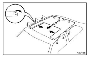
(b) Remove the roof headlining.
