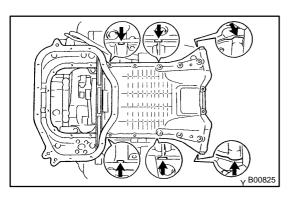
(b) Using a screwdriver, remove the No.1 oil pan by prying between the oil pan and cylinder block in the sequence shown.
