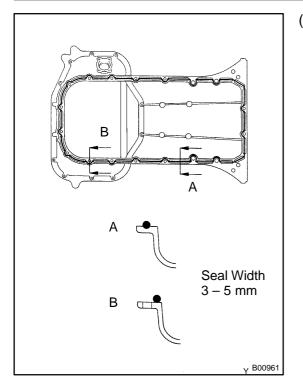
(b) Apply seal packing to the No.1 oil pan as shown in the illustration.
