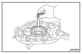
3. **INSPECT ROTOR TIP CLEARANCE**
