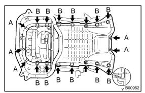
(c) Temporarily install the No.1 oil pan with the 17 bolts, stud bolt and 2 nuts.
