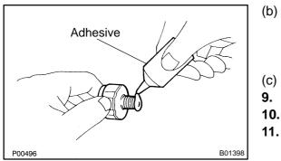
(b) Apply adhesive to 2 or 3 threads of the oil pressure switch. Adhesive:
