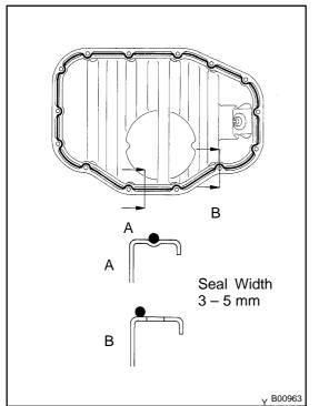
(b) Apply seal packing to the No.2 oil pan as shown in the illustration.
