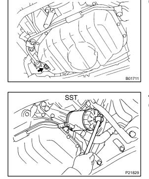
(b) Remove the oil drain plug, and drain the oil into a container.
