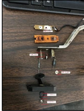
Figure 7. Reed Switch System
