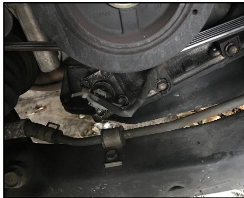
Figure 1. Oil Level Sensor Location
