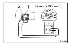
(2) Place the transmission in gear and while running at about 62 mph (100 km/h), measure the voltage between ECU terminals 2 and 6.
