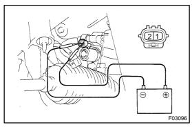
(c) Check the PPS solenoid operation.
