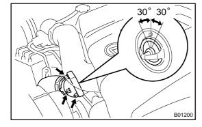
(b) Insert the thermostat into the water inlet housing with the jiggle valve facing straight upward.
