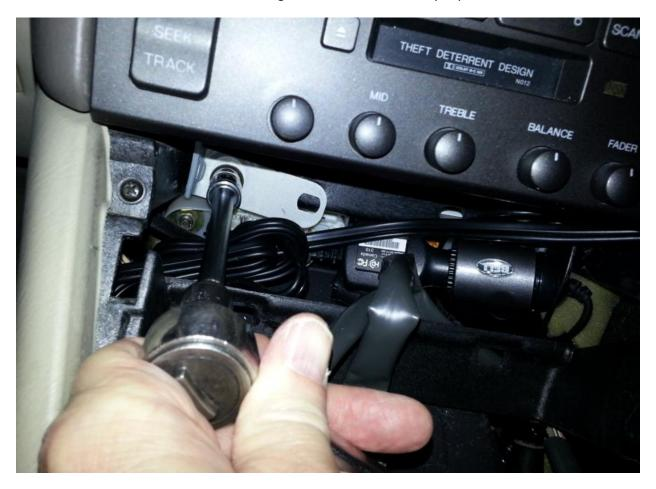
Use a towel to protect the vinyl on the console rails. Pull the radio/HVAC unit out and rest it on the towel.
