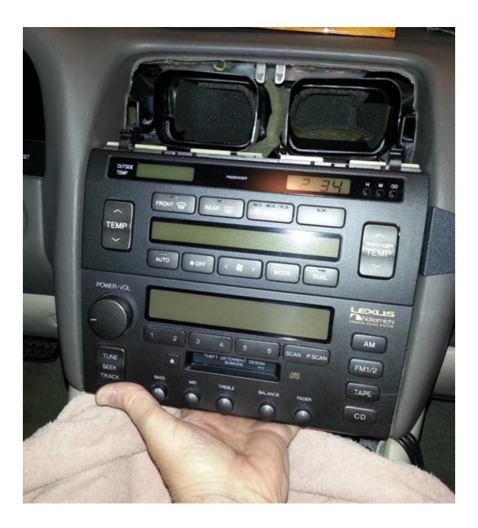
Unplug the radio and HVAC connectors from the radio/HVAC assembly.
