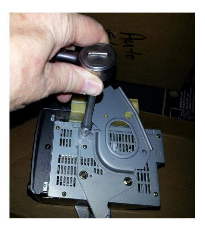
Separate the radio head unit from the frame.
