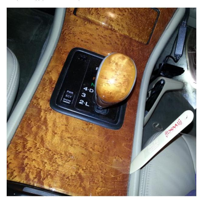
Remove the wood console panel. Disconnect the connectors for the ashtray light, VSC, seat heater switches, etc. Set the wood console panel aside.
