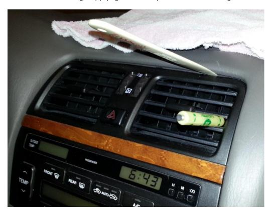
Slide the vent assembly out, move the hazard flasher connector, and set the vent assembly aside.
