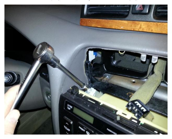
Remove the two bottom 10mm bolts holding the radio/HVAC assembly in place.
