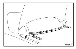
(b) Using a scraper, pry off the moulding from the 6 clips and remove the moulding.
