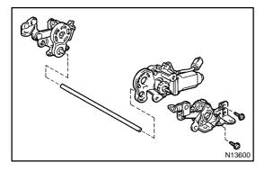
(c) Remove the inner front vertical sub—assembly, outer front vertical sub—assembly, front vertical motor and front vertical connecting pipe.
