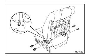
(d) Remove the 4 bolts and seatback assembly. Torque: 18 N-m (185 kgf-cm, 13 ft-lbf)
