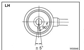
(b) Using SST and a press, install a new cushion as shown in the illustration.
